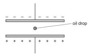
The potential difference across the plates is *V* and the separation is *d*.
